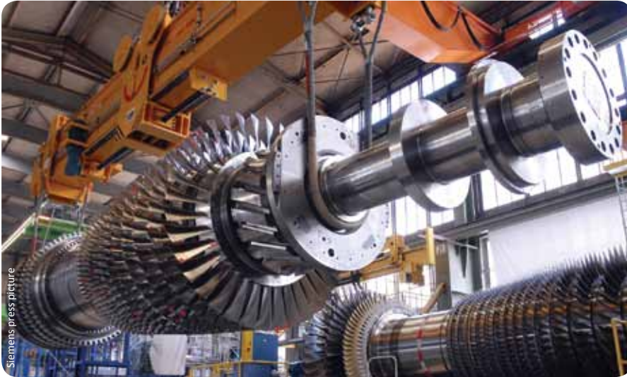
This 375-megawatt Siemens gas turbine, in use since December 2007 at the Irsching power plant near Ingolstadt, Germany, is a record-breaker. In association with a steam turbine, it can reach efficiencies of over 60% and satisfy the power needs of more than 3 million residents.
